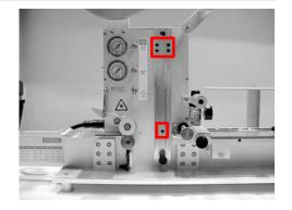
**Caution:** Line up the sealer connector pins with the sealer receptacle holes **before** tightening them together. If they are not lined up, serious damage could occur to the sealer.
